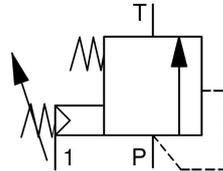
*The valves work pressure balanced and they are inserted in bypass.
